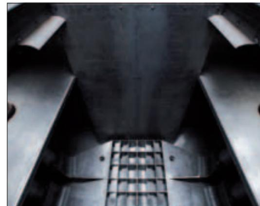
However, it is precisely these steels with reduced hardenability (i.e. low-alloy or non-alloy steels) that require a short steam-layer phase if optimum hardness is to be achieved. It is therefore important to use a high-speed flow of oil to disintegrate the insulating film of steam as quickly as possible. Flow rate also has a decisive influence on correct hardness during the subsequent boiling phase, when the oil begins to bubble up.
